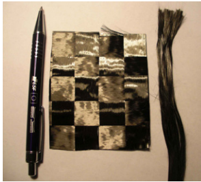
Fig. 1. Structure of the carbon fabric and the carbon fiber.
