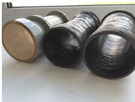
Fig. 4. View of the antennas made of metal (left), carbon fiber and carbon fabric (right, respectively).
