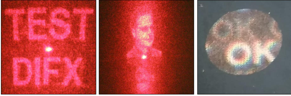
Fig. 4. a), b) Photos of the image recovered from the “hidden image” CGH on a scattering screen. c) Photo of the photoresist surface with the “text in lens” CGH element.
